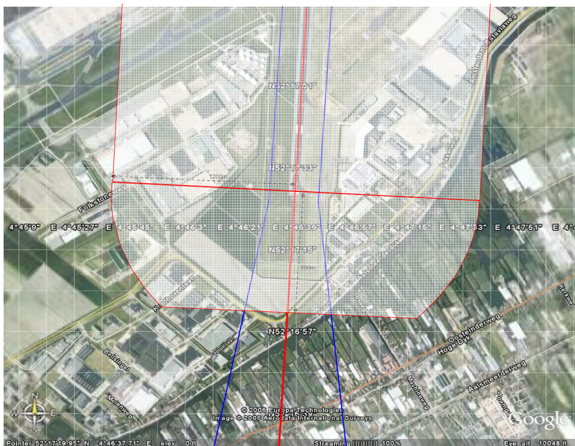
Figure 8-4: Area around runway 36R of Schiphol Airport where more stringent limitations than approved by Annex 14, should be applied to obstacle heights
