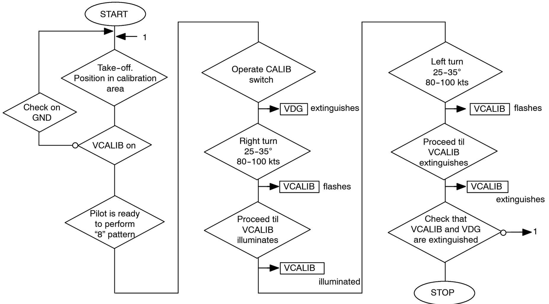
**Magnetic Sensor Calibration Unit, Connectors EC 135, BK117 C-2**
